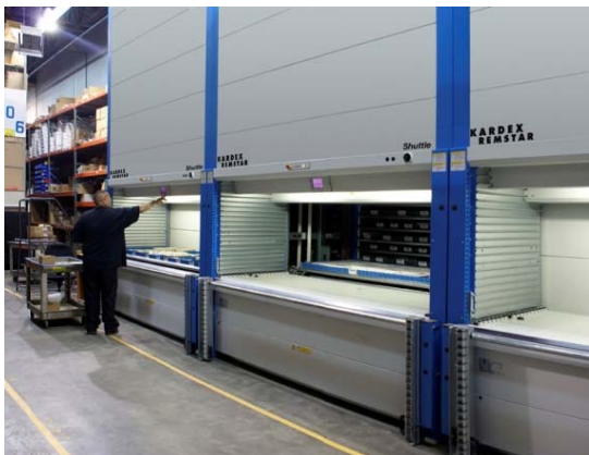
FIGURE 2B, three VLMs are arranged in one pod with one operator picking from all three VLMs.
