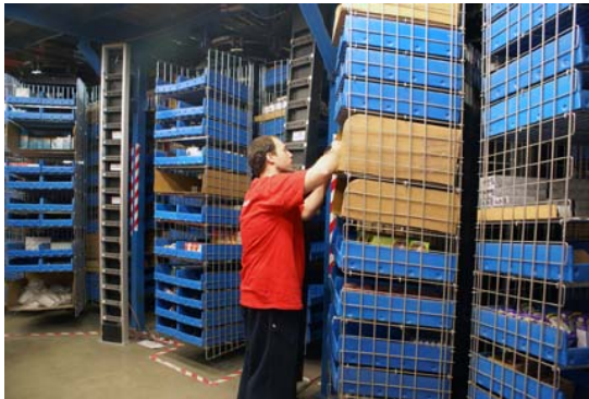
FIGURE 2A, four horizontal carousels are arranged in one pod with one operator picking from all four carousels.
