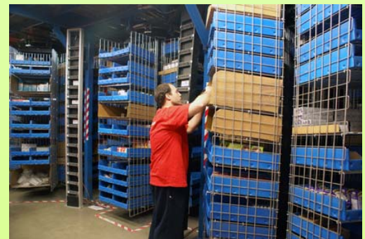
Six horizontal carousels are stacked to create two zones of three carousels each.
